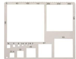
could tally the stones based on size class). The gravelometer provides a more accurate measurement of pebble/rock being measured.
